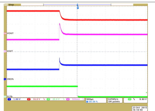
R_{\text{ILIM}} = 12 \text{ k}\Omega MODE pin connected to RTN Load transient event from 37 \Omega to 15 \Omega
